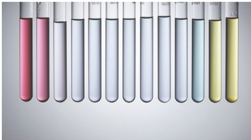
■ Figure 23.222 The colour changes observed with an anthocyanin indicator extracted from red cabbage as the pH is increased from low pH (left) to high pH (right)
