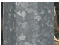
■ Figure 22.21 The grains of zinc on a galvanized lamp post can be seen clearly
