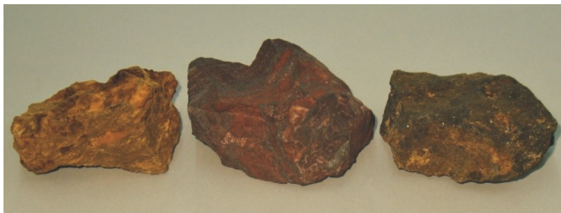
■ Figure 22.15 Samples of the major iron ores. a limonite, b hematite and c magnetite
