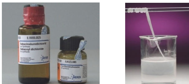
■ Figure 22.117 a The monomers for the 'nylon rope' experiment (decanedioyl dichloride [or sebacoyl chloride] and 1,6-diaminohexane); b the 'nylon rope' can be continuously drawn off from the interface between the solutions of the two monomers. This experiment produces nylon-6,10
