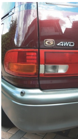
■ Figure 22.58 Car bumpers can be made of the isotactic form of poly(propene)
