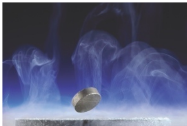
■ Figure 22.96 The Meissner effect: the floating magnet is only in contact with air
